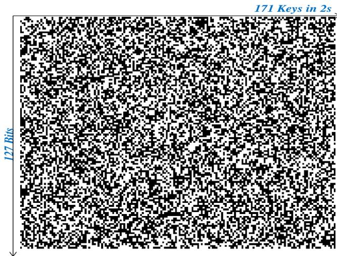
Figure 14: Key bits after quantization (WiFi, 2462 MHz , indoor NLOS)
