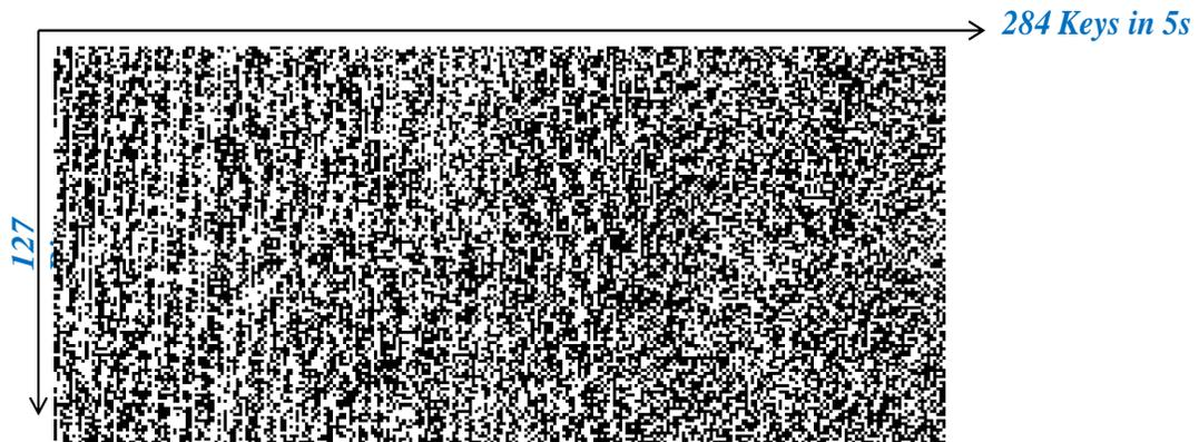
Figure 10: Key bits after quantization (LTE, 2627.5 MHz, outdoor urban street)
