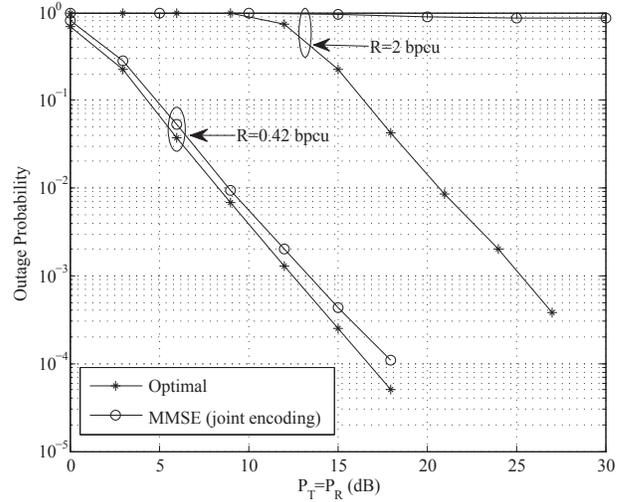
Fig. 3. Outage probabilities of  $2 \times 2 \times 1$  MIMO AF relaying systems with  $R=0.42$  and 2 bpcu
