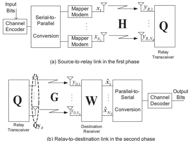
Fig. 1. Joint encoding/decoding structure for MIMO AF relaying systems with linear MMSE transceivers
