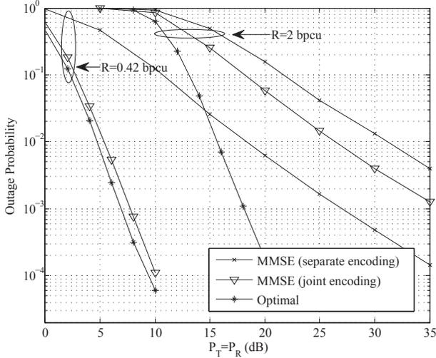
Fig. 2. Outage probabilities of  $2 \times 2 \times 2$  MIMO AF relaying systems with  $R=0.42$  and 2 bpcu
